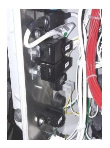
Caution: Do not remove contactor command relays (PSCONR, GENCONR, CCONR and HTCON1R) on units before the serial number stated if you fit new Electronic Contactors
